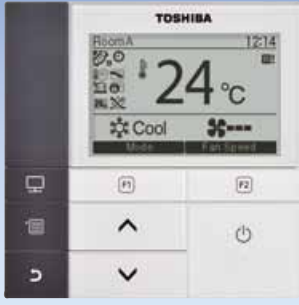
Wired Controller RBC-AMS51E-EN • Backlight • Weekly schedule
